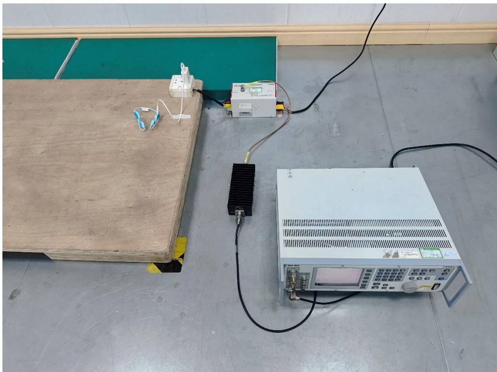
Photograph 8: Setup for Radio-frequency continuous conducted (CS), AC mains
